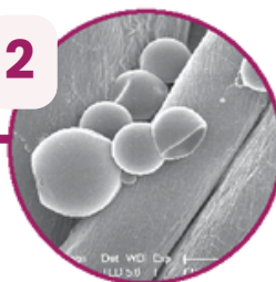
2 The microcapsules attached to the fiber release the Hyaluronic Acid on the skin surface
